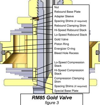
16 **Install the Piston Ring Energizer O-ring** (supplied in the kit) onto the Gold Valve Shock Piston. Do not re-use the stock oring. Be sure the o-ring sits all the way down into the groove and install the new piston ring.
